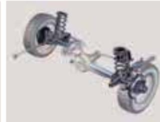
The heavy-duty coil spring suspension, incorporating telescopic shock absorbers and a torsion bar, provides confident handling.
